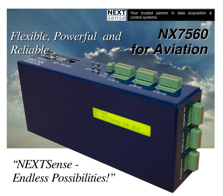
The NEXTSense NX7260 is an intelligent data logger that offers a complete set of acquisition, processing, logging and dissemination features. It is designed especially for automated weather stations – where system reliability and flexibility are important.
